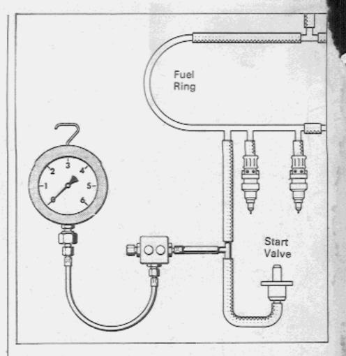
Before testing the system for correct pressure value, remove the pressure regulator vacuum hose at the regulator or manifold and block the opening (see Fuel System Description). Start the engine and let it idle. Read the gauge for the correct pressure as shown in the Test Chart: 2.2-2.6 bar. Now reconnect the vacuum hose to the regulator. The pressure should drop to about 2 bar at idle, and rise again when the throttle is opened. If this is not the case, check the vacuum hose for leaks.
