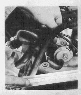
thermo-time switch is tested in the vehicle r correct resistance values at certain engine emperatures as given in the Test Chart. For this purpose remove the plug from the switch and measure directly at the terminals of the switch The illustration below shows the condition of the thermo-time switch when the coolant temperature is below 50°F: terminal W is connected to ground to complete the circuit and activate the cold start valve.
