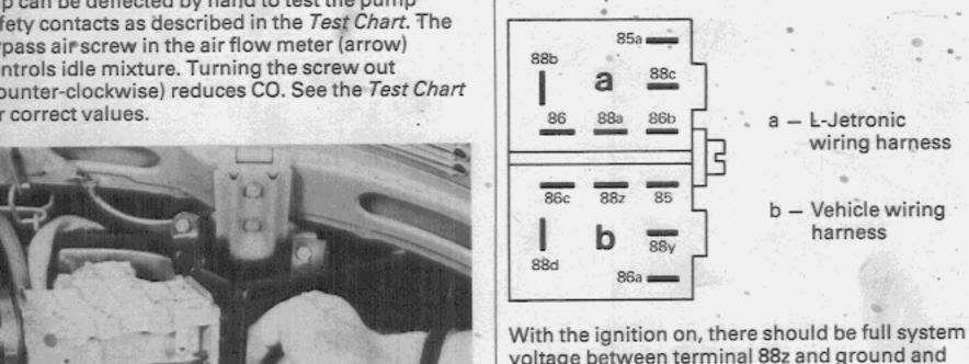
voltage between terminal 88z and ground and between 88b and ground. If this is not the case, the relay is defective.
