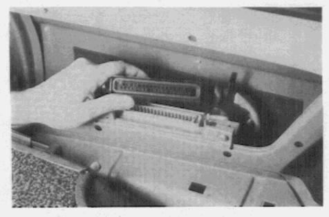
The wiring harness plug is removed from the ECU for many of the tests described in the Test Chart.
